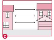
Provide greater spatial separation between structures in hazard areas to limit the spread of fire from one structure to another.
