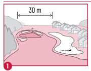
Integrate minimum 30 m wide zones (fire breaks) featuring ignition resistant materials (e.g., mowed grasses, ponds, roads) into community design to limit the spread of fire. Increase minimum to 50 m on steep slopes.
