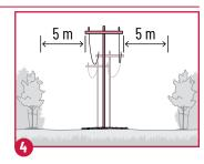
Design/update structures and infrastructure to be ignition resistant (e.g., 5 m distance between vegetation and power lines, power supply lines below ground where feasible).
