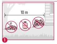
Complete regular maintenance of structures, infrastructure, and landscaping within 10 m to limit accumulation of flammable materials (e.g., leaves, brush piles, stored items, fuel tanks).
