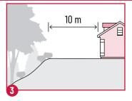
Require minimum 10 m setback from the crest of a hill to limit spread of fire to structures.
