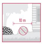
Remove combustible materials (firewood and lumber) stored within 10 m of house perimeter and under decks.
