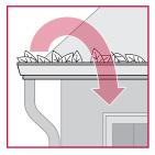
Remove needles, leaves and other debris from gutters, roof surfaces, decks and balconies. Regularly clean vents.
